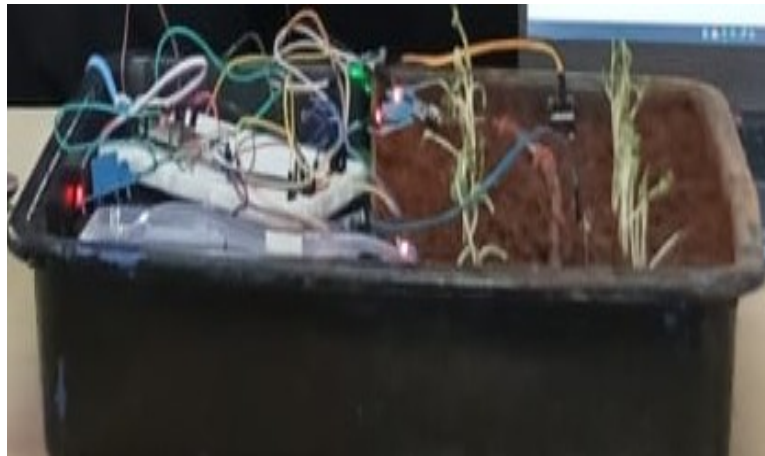
Figure 4.3: Final Working Model of Smart Irrigation System
